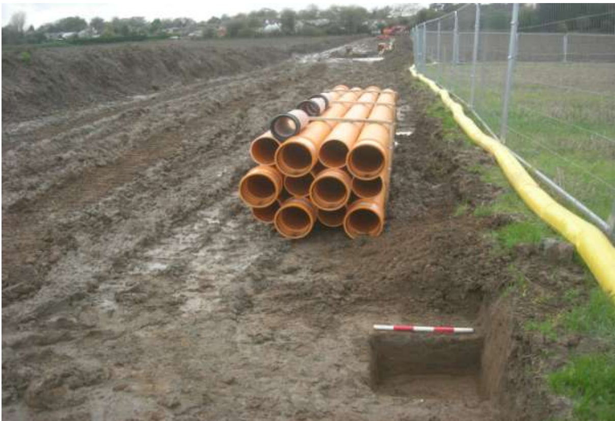
Plate 2. Test Pit showing depth of topsoil and subsoil. Plate 3 (below) Test Pit showing depth of topsoil and subsoil.
