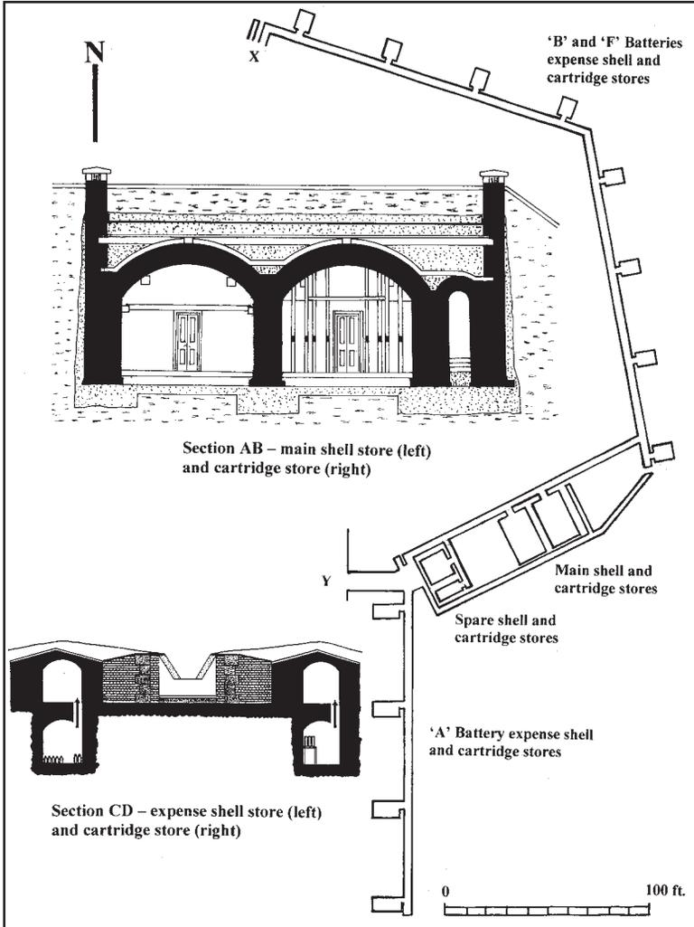
Fig. 5 Plan of the magazines as built in 1868-72, with cross-sections.
