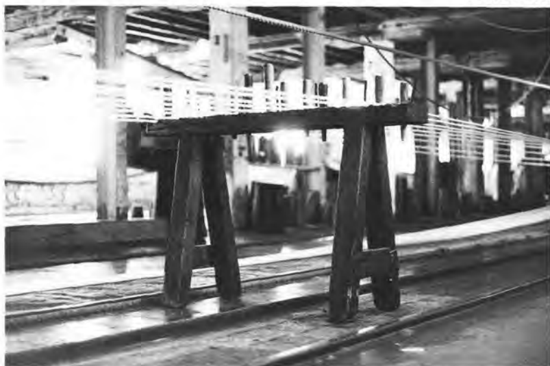
A trundle used to support and separate the yarn and strands during the processes of combining and closing
