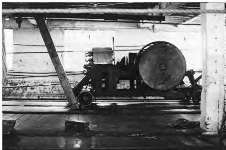
One of the heavier jack wheels brought into the yard during the mid-1850s. Unlike its lighter predecessor, it was designed to run on rails
